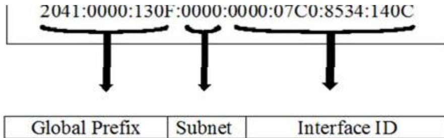
Fig. 1. IPv6 Address Format
