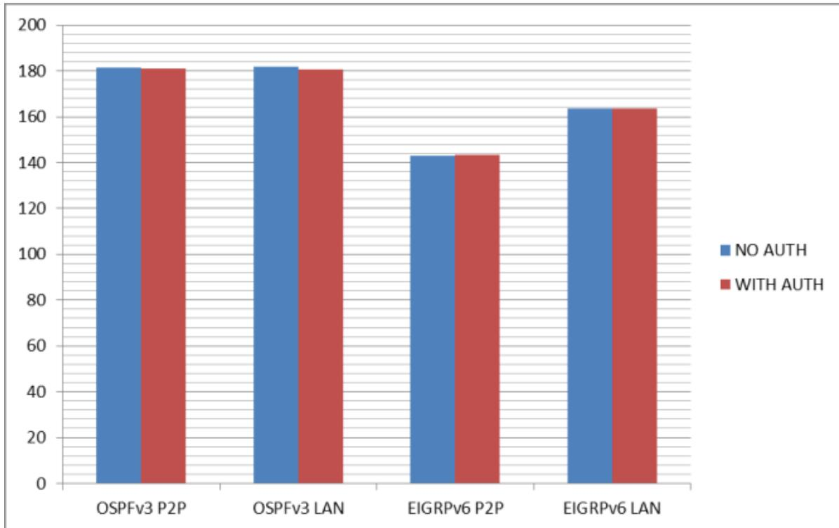
Fig. 5. EIGRPv6 and OSPFv3 Cold Start-up Time Comparison
