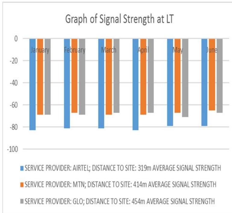
**Fig. 2. Graph of signal strength at LT**
