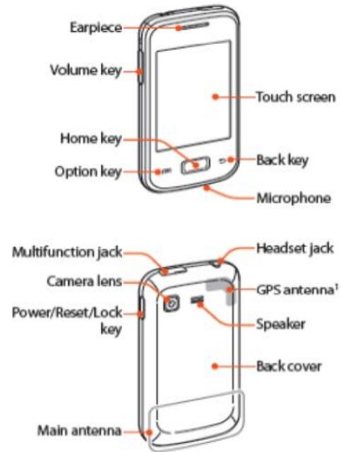
Fig. 1. Front view of the mobile device
