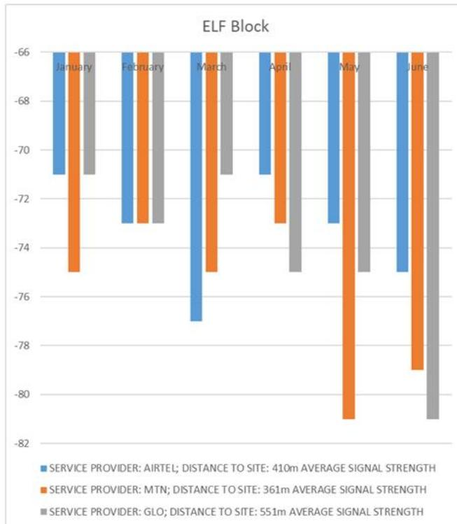
**Fig. 7. Graph of signal strength at ELF block**
